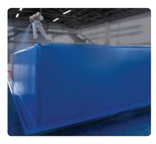
The chemically formulated coloured gel coat specifically for swimming pools is meticulously applied to the surface of your swimming pool.
